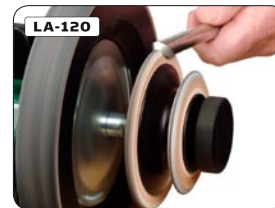
LA-120 Profiled Honing Wheels For honing the flutes. One radiused and one pointed.
