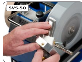
SVS-50 Multi Jig For skewers of any shape, even with an oval section.
